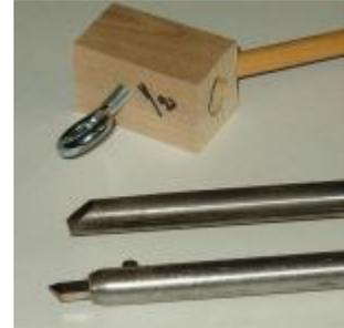
Here is a 60 degree holder and the typical spindle gouge grind it gives. I did not mark the gouge size on the holder as I seldom use spindle gouges and use this holder for 1/4" to 1/2" spindle gouges. I could do the same for the bowl gouges or Oland tools but prefer to have one for each size shaft as I use the Oland tools a lot and am too lazy to want to keep turning the eye bolt in and out.
