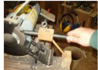
Normally I sharpen a skew by hand but if you are new to sharpening the jig can be used. Note that the long point will have a longer bevel than the short, but this does not hurt the cutting with the skew.
