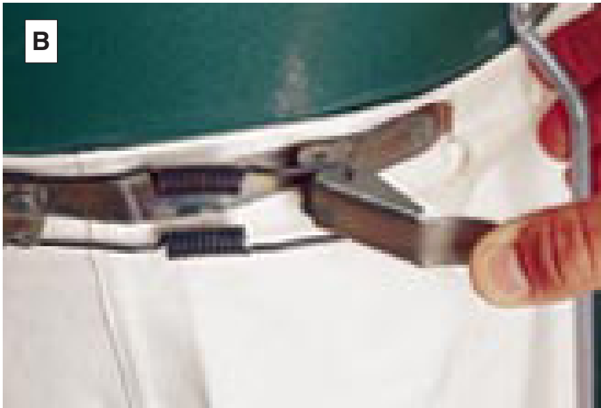
B The release lever on the Grizzly G8027's bag clamp bent easily when closing it. Since our test, a Grizzly spokesman told us they would improve the clamps.
