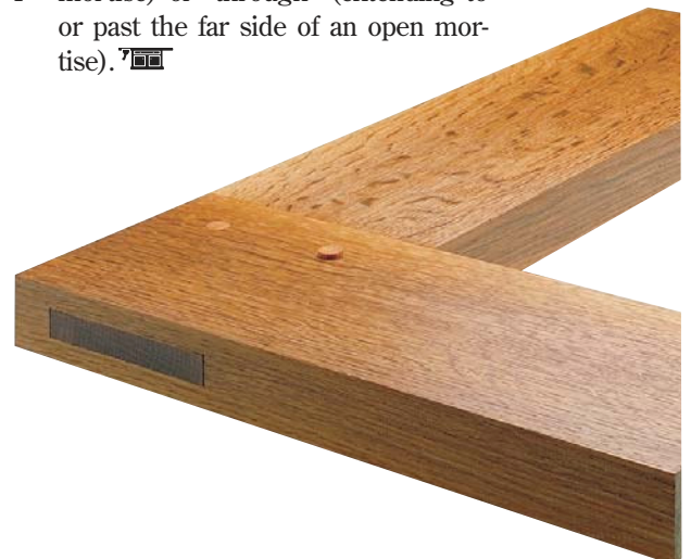
6 Use a clamp to close the joint, then check the assembly for square. Drive the pegs with a deadblow or wooden mallet.
