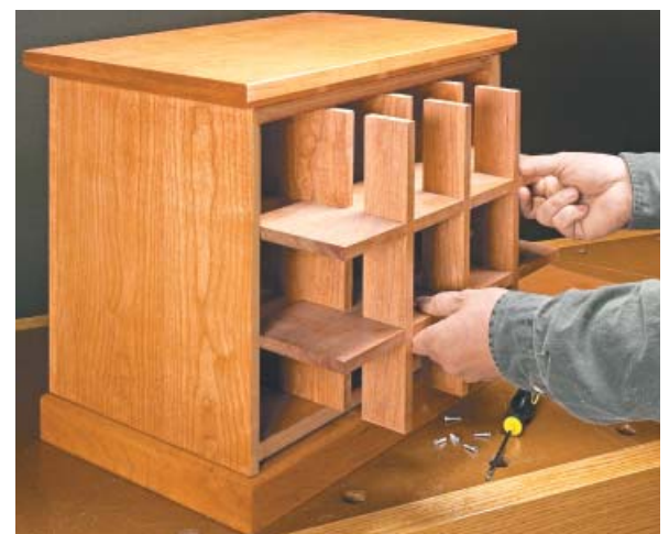
▲ Installing the Dividers. Since the dividers are not glued together it's easy to apply the finish. And after assembly, they slide straight into the case from the back.
