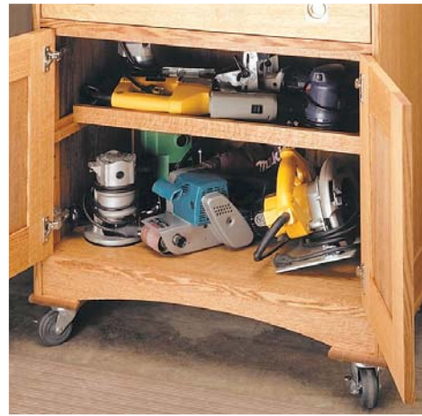
B. Shelf & Tray. Portable power tools are stored underneath on a large bottom shelf and a sliding tray.
