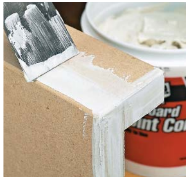
▲ Edge Sealer. Drywall joint compound makes a quick, easy sealer for the porous edges.
