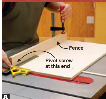
Square the fence to the end of the base and secure the free end with a clamp.
