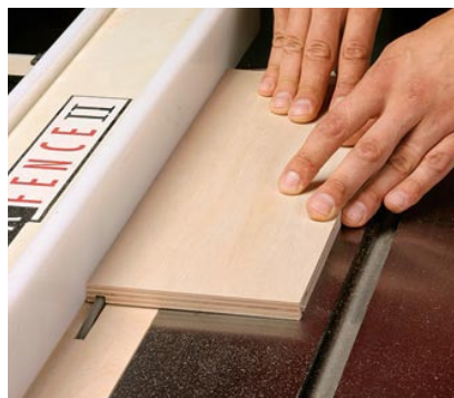
Grooves for the bottoms. Run the bottom of the sides, fronts, and backs against the fence to cut the groove for the bottom panel.
