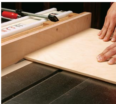
Rabbit the bottom panels. All four sides of the bottom panels are rabbeted to fit into the grooves running around the bottom of the drawer box.
