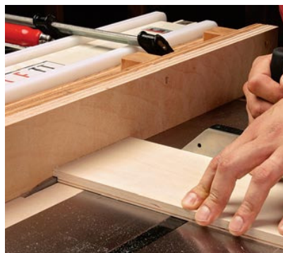
Rabbit the fronts and backs. With the dado head buried in a sacrificial fence, cut the rabbets for the corner joints.
