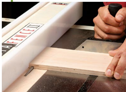
Dados in the sides. Use a miter gauge to guide the drawer sides safely along the rip fence.
