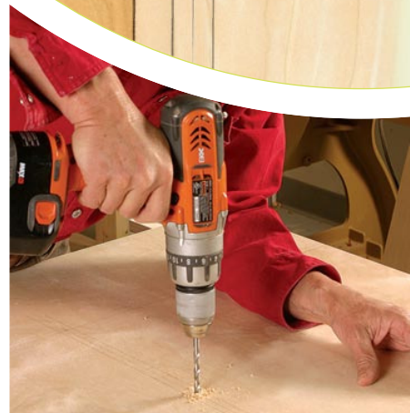
Drill along the centerline. Two lines show the edges of the intersecting panel. The third line marks the centerline for the clearance holes.
