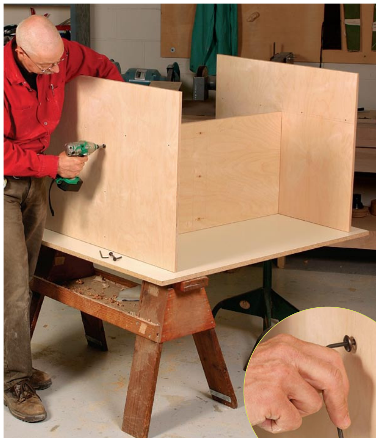
Use a drill to start the screws. Drive in the joint-connector bolts, leaving them about \frac{1}{8} in. proud of the panel.
