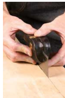
A jig such as the Veritas Variable Burnisher allows you to turn a hook with little chance for error. If you are having difficulty with burnishing freehand, this is an excellent option.
