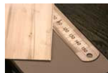
The ruler trick sharpens the scraper only at its cutting edge, saving much time and effort.
