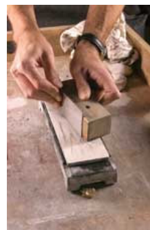
There are many ways to stone an edge. This 2" x 2" x 5" block is what I prefer. You can move the block as you rub the scraper against the stone, which spreads the wear out on your stone. Alternately, with thick waterstones you can use the side of the stone and support the scraper with a block of wood.
