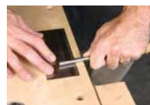
Rub your burnisher flat against the scraper five or six times. This work-hardens and consolidates the material. And it draws out the steel at the edge, making it easy to turn the hook.
