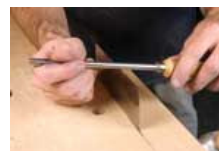
Burnishing freehand is tricky for some and a cakewalk for others. Here's a tip: Rest one hand on the bench to control the angle of burnishing. Use the other hand to draw the burnisher along the edge of the scraper. This usually helps increase your control.
