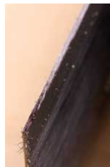
After two strokes with the file, the color is almost gone from the edge.
