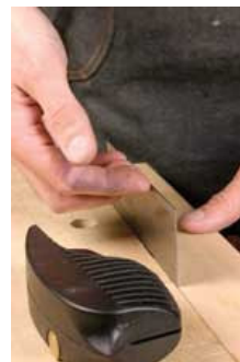
After three passes with the burnisher using mild downward pressure, feel the edge for a hook as shown. It should feel like a tiny lip that your fingernail could almost grab.
