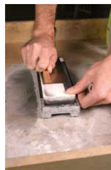
Hold the ruler with one thumb or it will slide. Use your other hand to stroke the edge against the stone. The wood block improves control.
