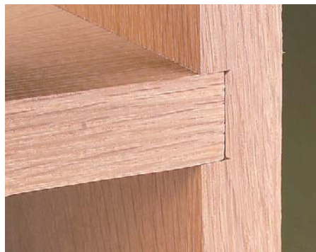
▲ Better. With stacked dado sets, the outside blades can leave score marks on the sides of the dado. While this doesn't weaken the joint, it's still noticeable.
