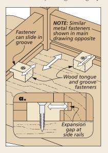
the top may crack or at the very least the joint will break and separate.
