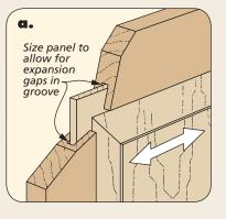
crossgrain movement in the door by confining it to a panel installed in grooves in a rigid frame.
